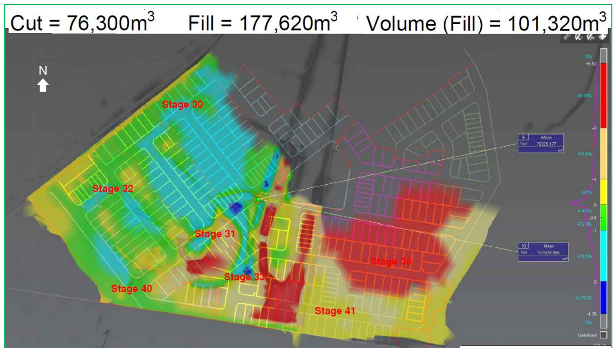
Figure 2: North Harbour Phase 4B Showing Bulk Earthwork and Layout Plan
